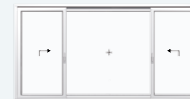
System K 2 lift/sliding sashes, 1 fixed pane
