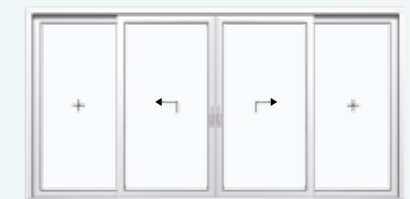
System C 2 lift/sliding sashes, 2 fixed panes
